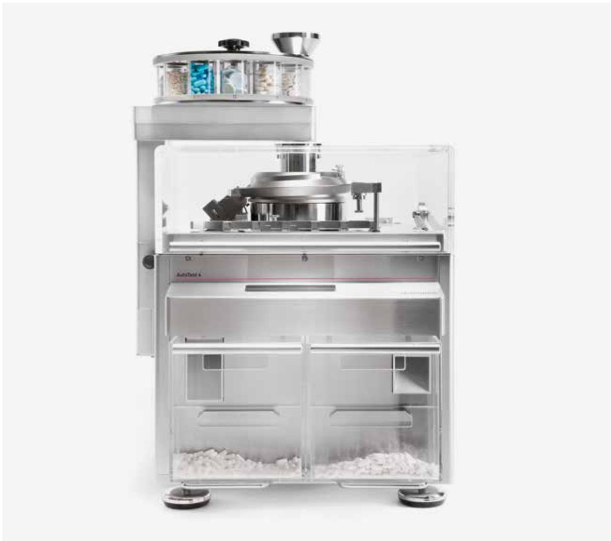
→ AutoTest 4 equipped with 12-magazine feeder
