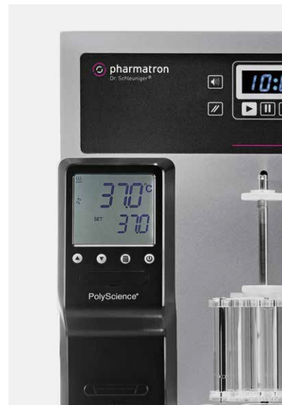
→ Immersion heater/circulator module with integrated temperature sensor
